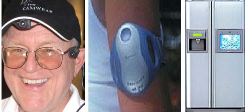
Figure 2 – Left: wearable video camera from Deja View. Middle: wearable bio-metric sensors by BodyMedia. Right: LG Internet fridge
